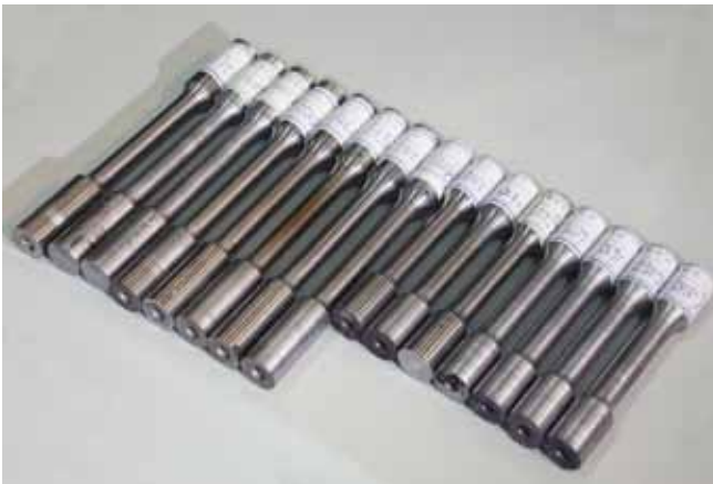
Precision Machined Test Bars in Accordance with ASTM A-370
