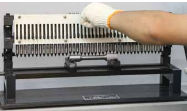
Profiling of Test Bars Prior to Tensile Testing
