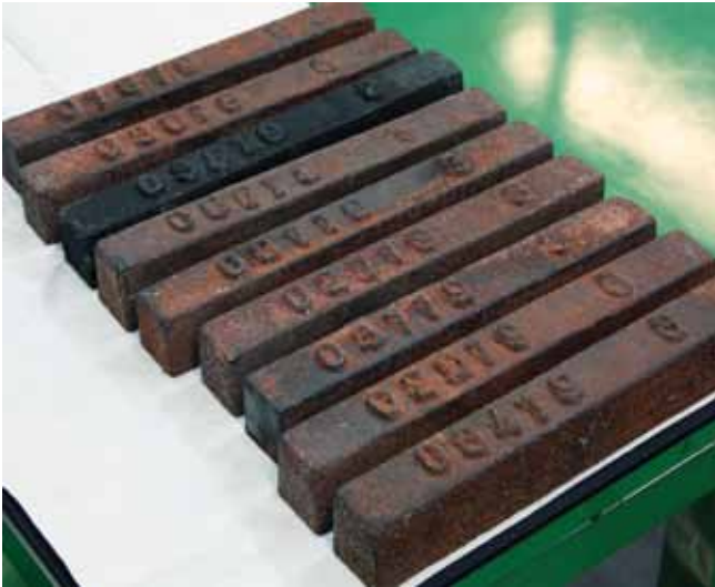
Cast Bars with full Traceability to Heat Numbers
